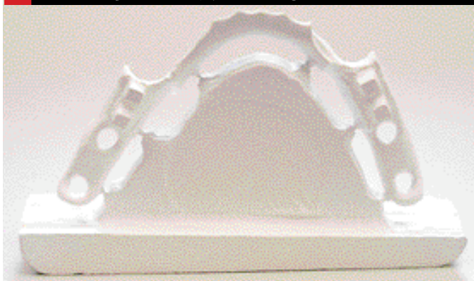
33 The milled plate is ready for sintering
