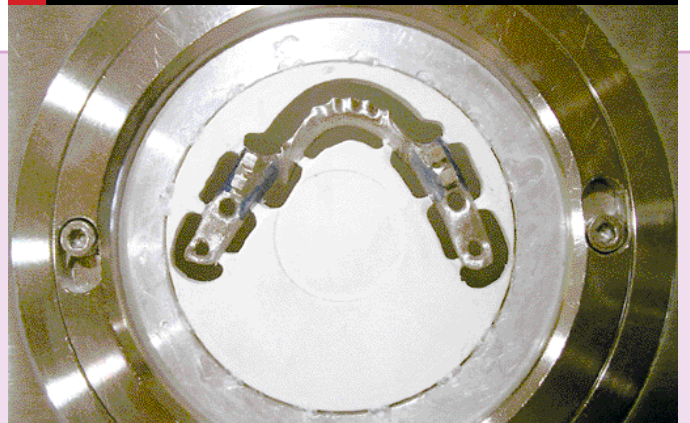
29 The palatine bar in the Zirkograph disc
