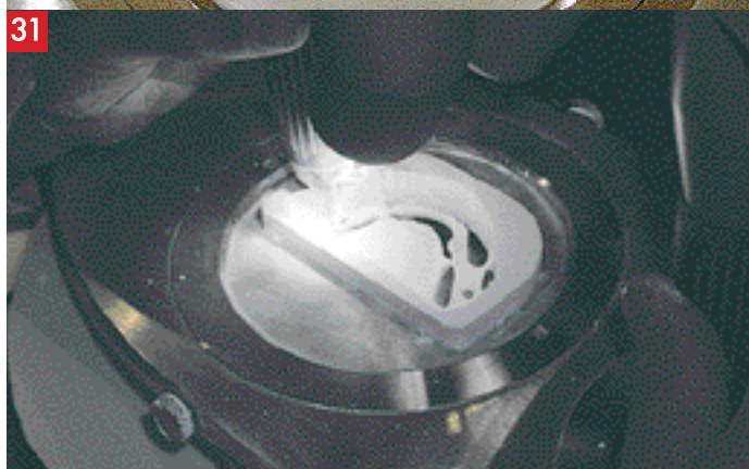
34 Figs. 34 and 35: Milling the secondary parts
